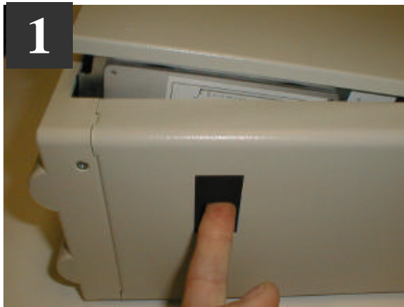
1 Open the Printer Top Cover by releasing the catch on the right-hand side of the printer.
